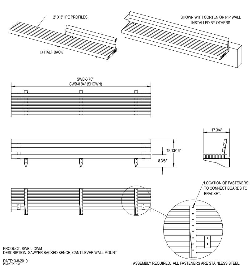
SITE FURNISHING IS POWDER COATED WITH TGIC POLYESTER. STEEL SURFACE PREP INCLUDES MECHANICAL AND CHEMICAL ETCHING FOLLOWED WITH A COATING TO IMPROVE ADHESION AND CORROSION RESISTANCE.
