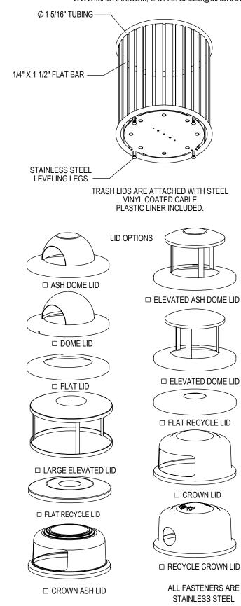
SITE FURNISHING IS POWDER COATED WITH TGIC POLYESTER. STEEL SURFACE PREP INCLUDES MECHANICAL AND CHEMICAL ETCHING FOLLOWED WITH A COATING TO IMPROVE ADHESION AND CORROSION RESISTANCE.
